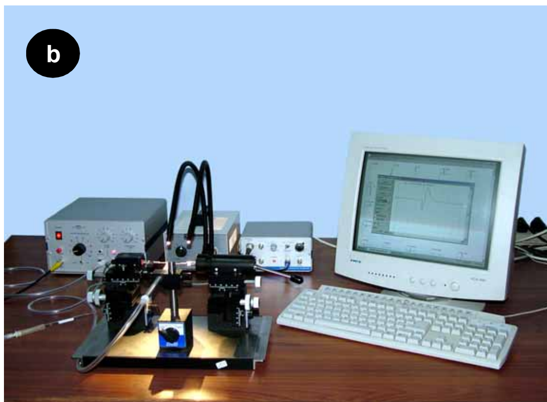
Plate 5. Instruments used for laboratory bioassay a. Wind tunnel apparatus b. Electro antennogram
