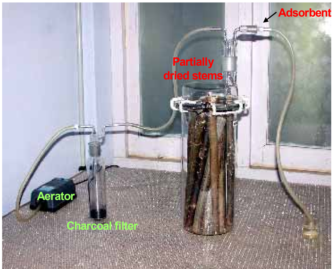
Plate 4a. Dynamic head space (DHS) volatile extraction unit.
