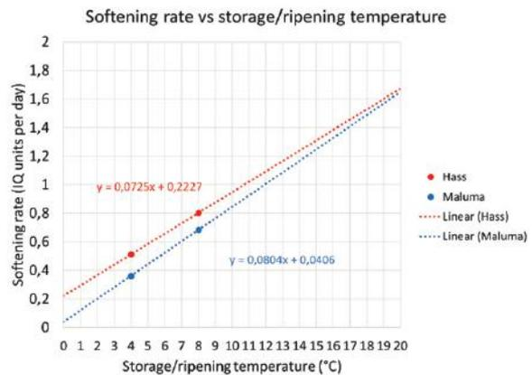
Figure 6. Extrapolation of the softening rates of 'Hass' and 'Maluma' fruit stored at, respectively, 4°C and 8°C.
