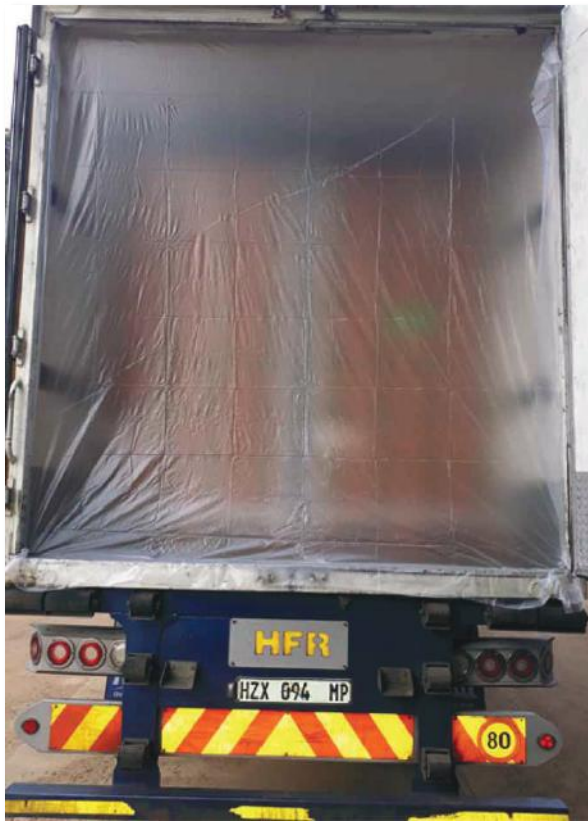
Figure 1. Curtain fitted behind the doors of a refrigerated truck from the service provider with the most air-tight trailers. The curtain was fitted to the inside of the trailer using double sided tape. Silicon was inserted in the corners.
