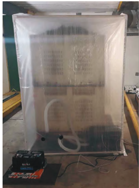
Figure 2. Tent and CO 2 controller assembly used in the packing house-based trials. The tent was designed for one pallet and consisted of a plastic sleeve fitted over an electrical conduit pipe frame. The controller-assembly was made up of a CPU unit housed in a plastic container. Plastic pipes were used to connect the valves to the plastic sheeting and the battery was placed on the outside of the tent.
