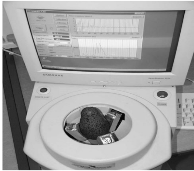
Figure 3: The Technion acoustic test apparatus "Firmalon".
