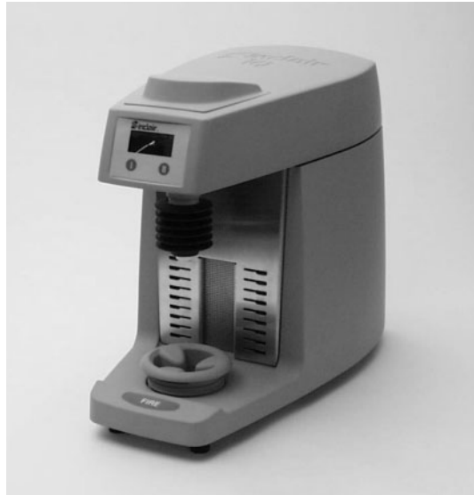
Figure 1: The Sinclair IQ™-FT low-impact testing apparatus.
