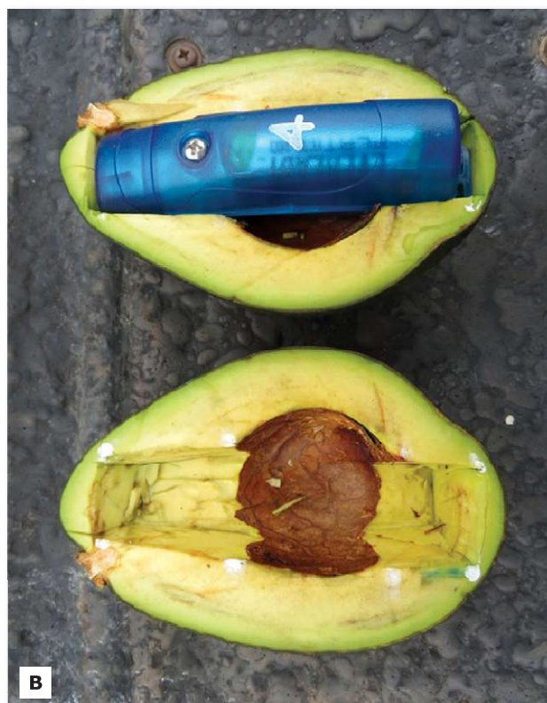
Figure 2: Accelerometer placement (A) on test vehicle as well as attached to a lug box and (B) embedded in avocado fruit
