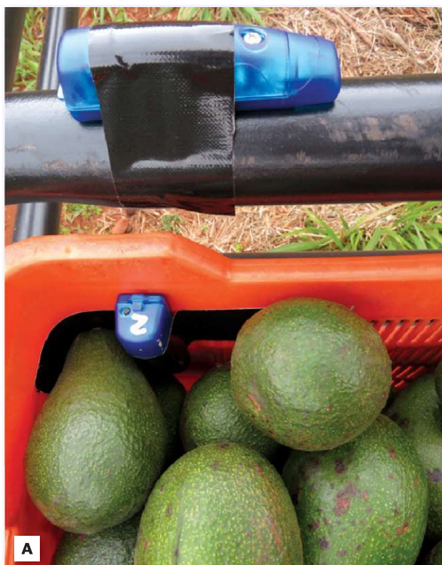
Figure 2: Accelerometer placement (A) on test vehicle as well as attached to a lug box and (B) embedded in avocado fruit
