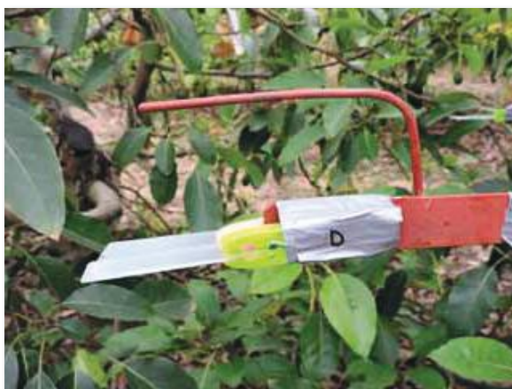
Figure 2. A spore trap with horizontally-held vaseline slides.
