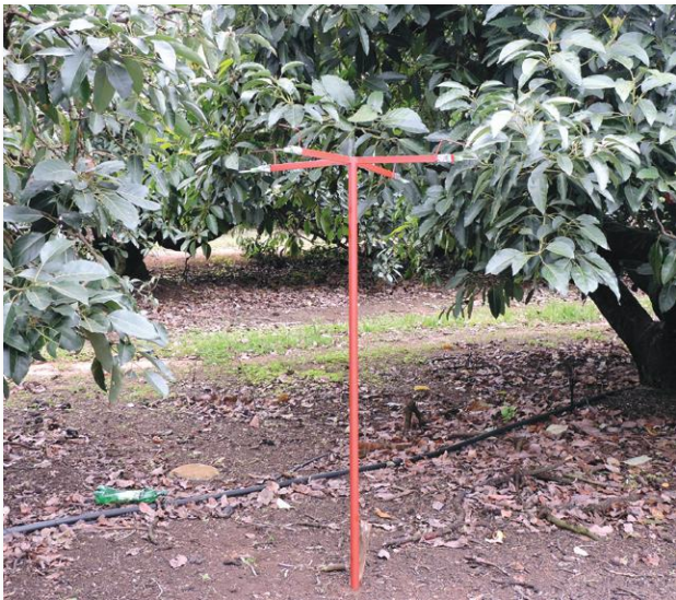
Figure 3: A spore trap with horizontal vaseline slides.
