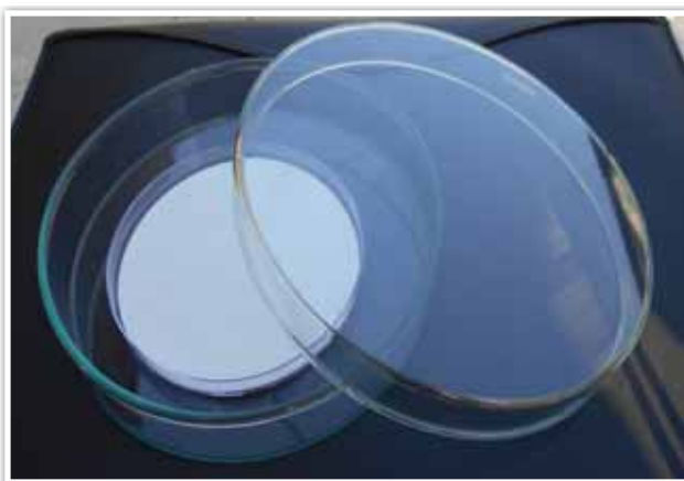
Figure 6. A modified White trap consisting of a Petri dish (85 mm diameter) placed in a glass Petri dish (140 mm diameter).
