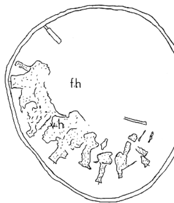
Figure 10. Diagram showing the bottom side of a disk cut from the trunk of a tree and repeatedly injected over a long period, indicating the distribution of discolored wood in a cross section: vh = discoloured, non-functional wood; fh = discolored, functional wood.
