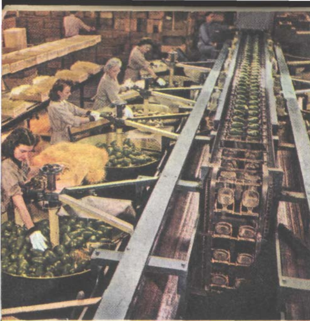
Fruit, moving on a conveyor belt, falls into bins according to size, is then crated and shipped out.
