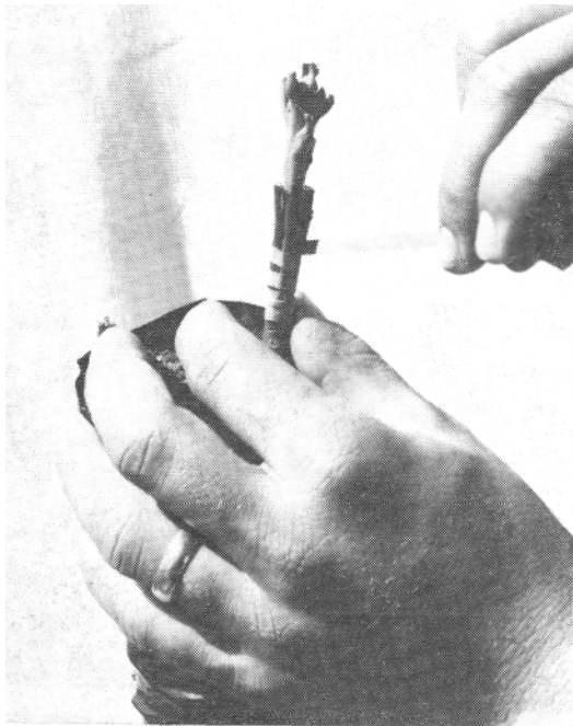
Fig. 2. Rubber strip used for wrap.
