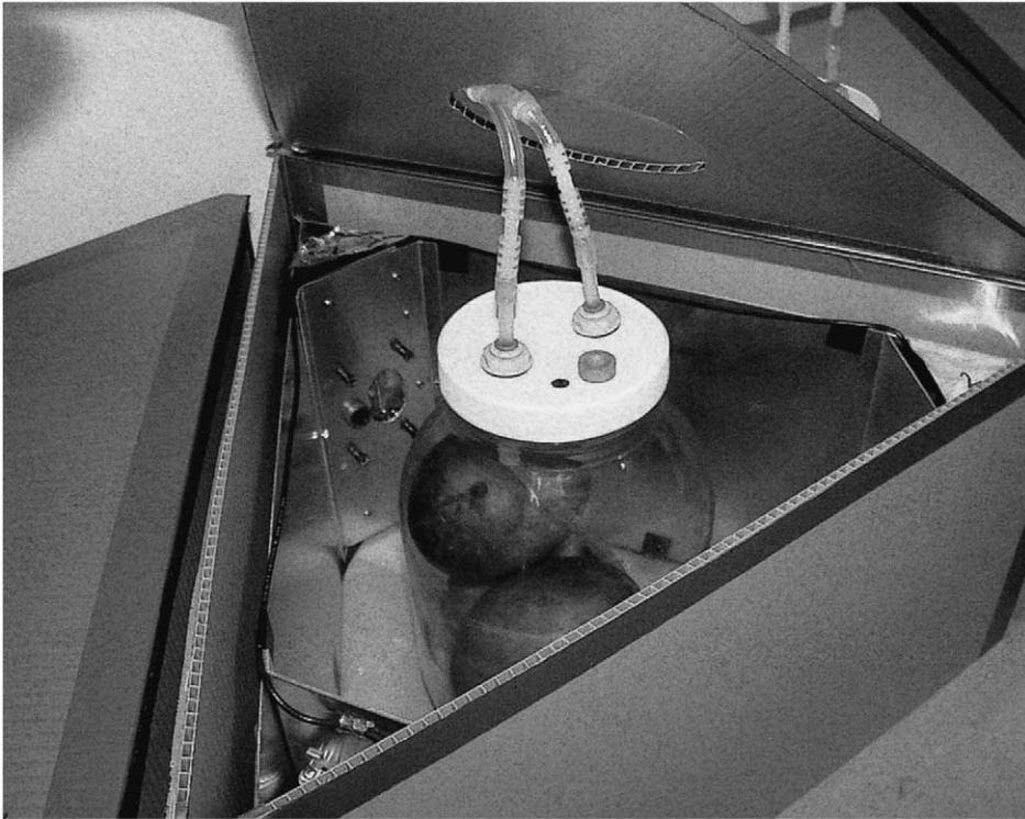
Fig. 1. One of the six triangular chlorophyll fluorescence sensor units with a sealed sample jar in the center containing mango fruit.
