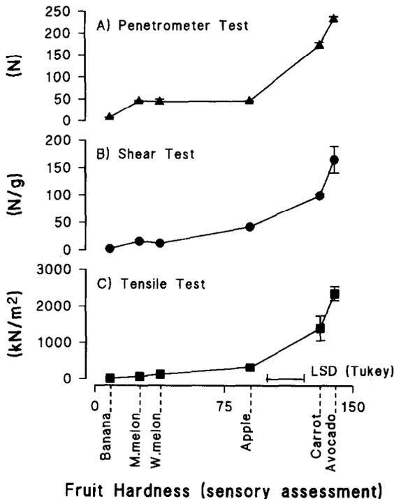
Fig. 3. Relationships between sensory assessment of fruit hardness and mechanical measurements of flesh firmness using a penetrometer (A), shear cell (B) and tension test (C). Points represent means of four measurements and vertical lines represent  $\pm$  S.E.M. (when larger than points).
