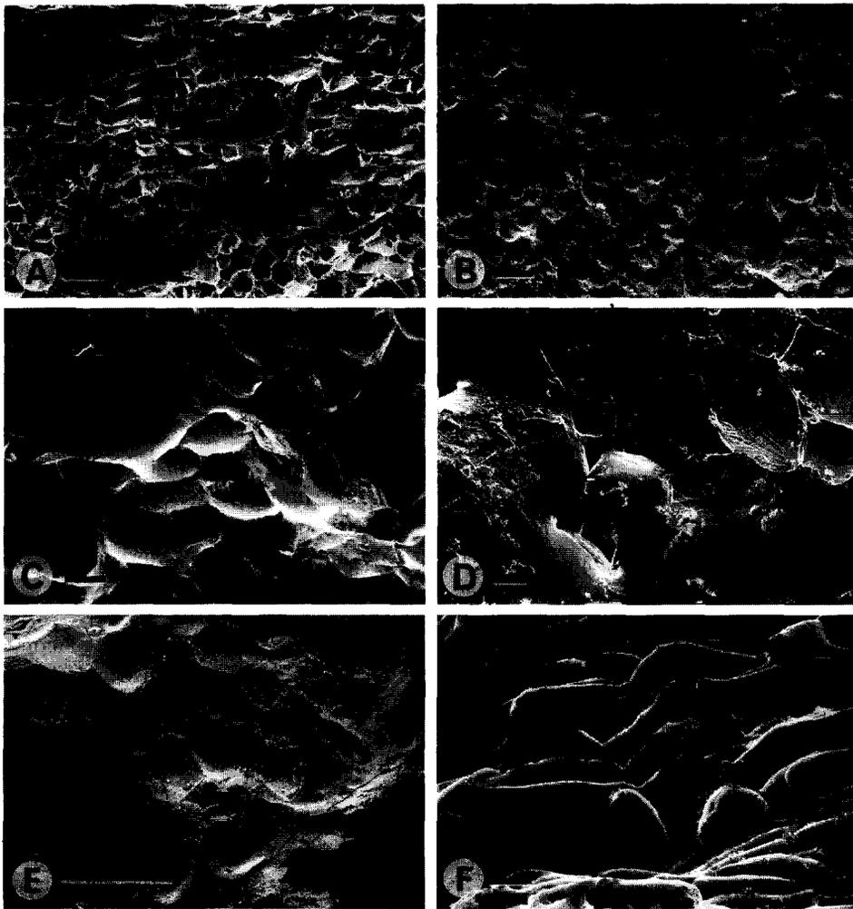
Fig. 2. Fracture surfaces of fruit tissue following tensile tests as observed using Low Temperature Scanning Electron Microscopy. (A) Carrot; (B) Avocado; (C) Apple; (D) Muskmelon; (E) Watermelon; and (F) Banana. Neighbouring cells have separated without breaking in banana, and muskmelon shows a mixture of broken and unbroken cells. The remaining fruit show breakage of all cells on the fracture surface. Bar = 0.1 mm (A, B, C, D, F); 1 mm (E).
