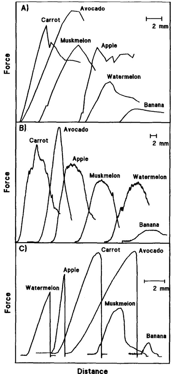
Fig. 1. Force-distance curves obtained during penetrometer (A), shear cell (B), and tensile (C) measurements of fruit texture. Curves are not plotted to scale. Respective maximum forces for banana, muskmelon, water melon, apple, carrot and unripe avocado are given in Fig. 3. Horizontal lines represent a scale of 2 mm.
