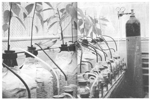
Aeration experiment with avocado seedlings. Compressed nitrogen gas and compressed air are led into 2-quart mixing which are connected by aeration tubes to the 20-liter bottles in which the avocado plants are growing.
