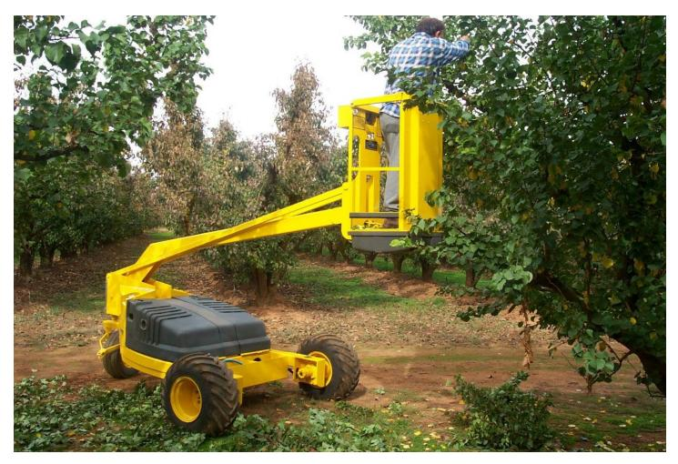
Single castor three wheelers are nimble and efficient for relatively flat areas– rated 5 to 7 degrees maximum
