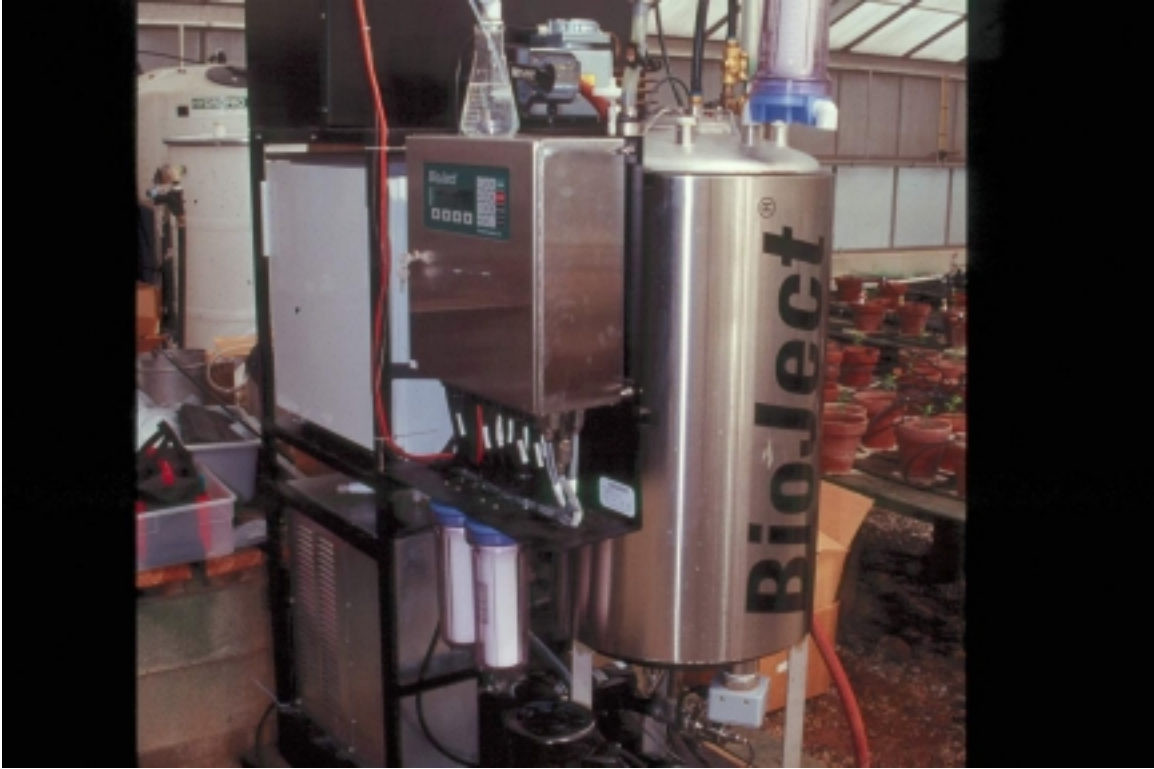
Fig. 3. Field fermenter used to produce biocontrol agents and continuously inject them into irrigation water.
