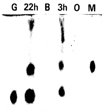
Fig. 2. Descending paper chromatography of products of avocado fruit pulp amylase activity. (G = glucose standard; h = hours; 0 = zero time; M = maltose standard; B = blank.)
