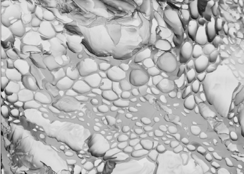
Figure 1. Magnification of biochar particle showing internal pore space that functions to increase water holding capacity, surface area, cation exchange sites, and as habitat for plant growth promoting bacteria and fungi.
