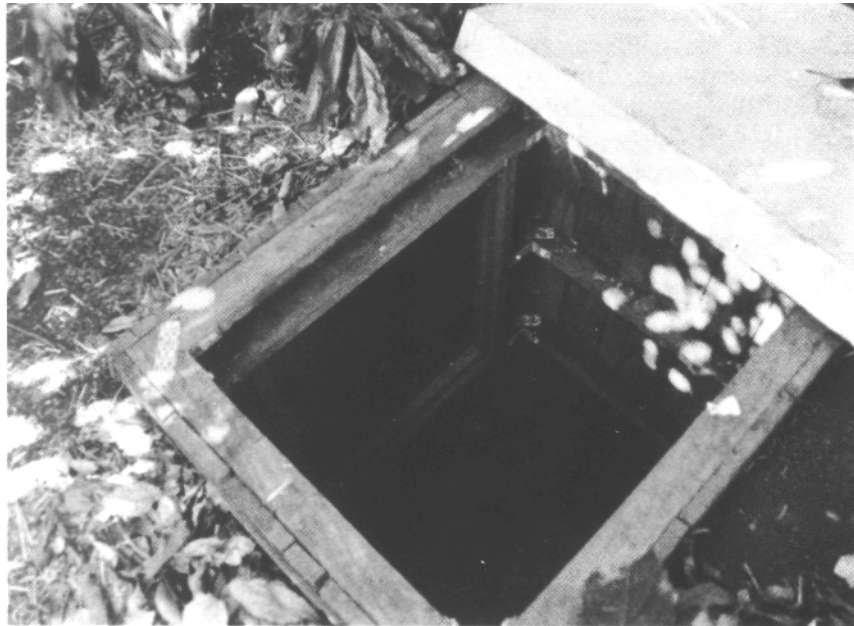
Fig. 3. Window to the roots. Rhizotron was installed by Whiley before trees were planted.
