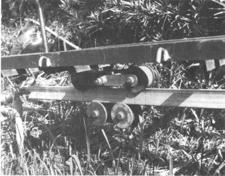
Attachment of trailer on rail with hard rubber rollers.
