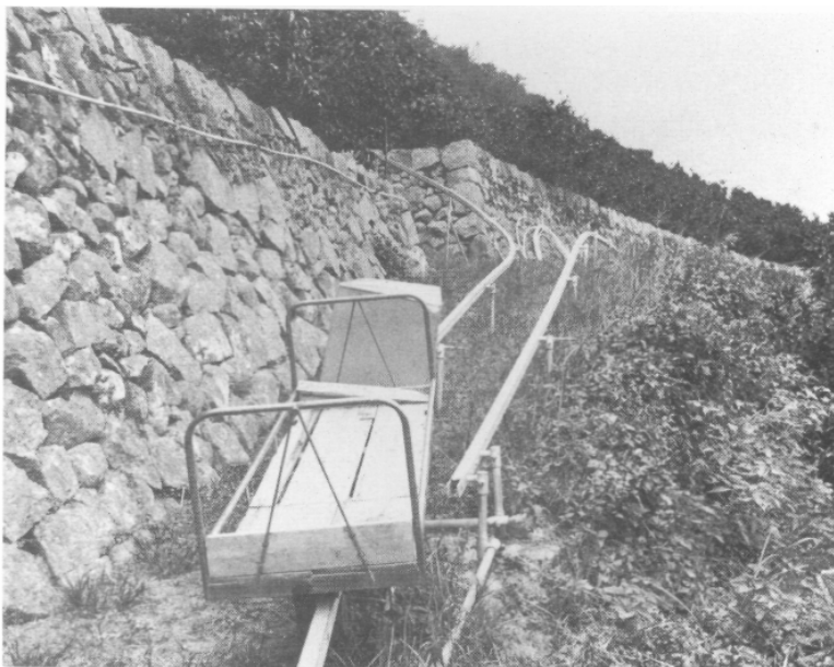
Two parts of same orchard can be serviced with the same power unit by changing short section of rail from one tract to another.
