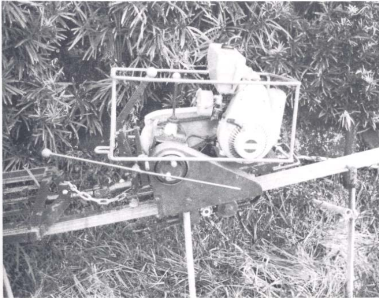
Another type of monorail system. Hard rubber roller engages shallow indentations on top of rail. Note trailer attachment, safety chain and guard rail around power unit.
