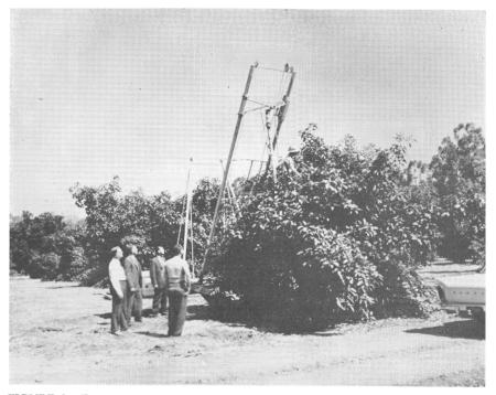
FIGURE 1. Demonstration of fruit picking machine by Dan Seamount, Assistant Specialist, Agricultural Experiment Station, Riverside. Mr. William Cowan and Mr. Phil Newman of Calavo, Gene Daggerman of Space Equipment Corporation, and Mr. Wally Wright of The Irvine Company are observing the test. The operator is shown with his swing seat swung to the left so that he may work directly up against fruit bearing branches.
