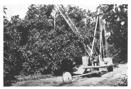
FIGURE 2. Dan Seamount is shown working within the branches of larger tree. The machine is self-propelled and self-guiding. The guide discs can be seen in the front center of the picture. The operator can lift himself up over and into the tree as he wishes.
