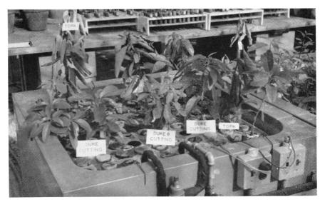
Fig. 1. Avocado cuttings and seedlings growing in temperature controlled tank containing nutrient solution, for root rot resistance tests.
