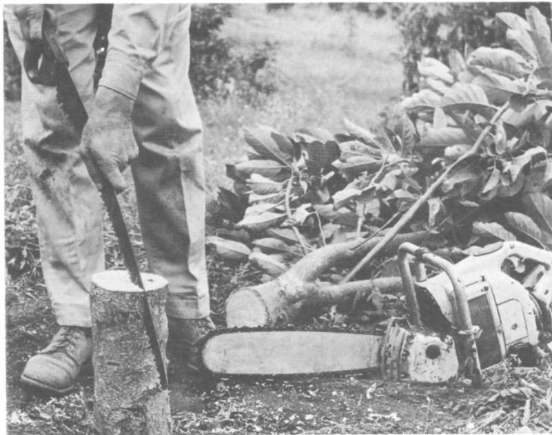
*Fig. 1. Two or more saw cuts are made, followed by notches in the edges.*
