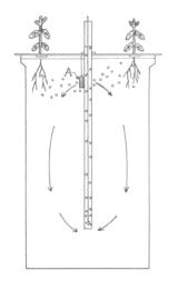
Fig. 1. Sketch of solution culture apparatus showing position of plant, aerator, and inoculum bag (A).
