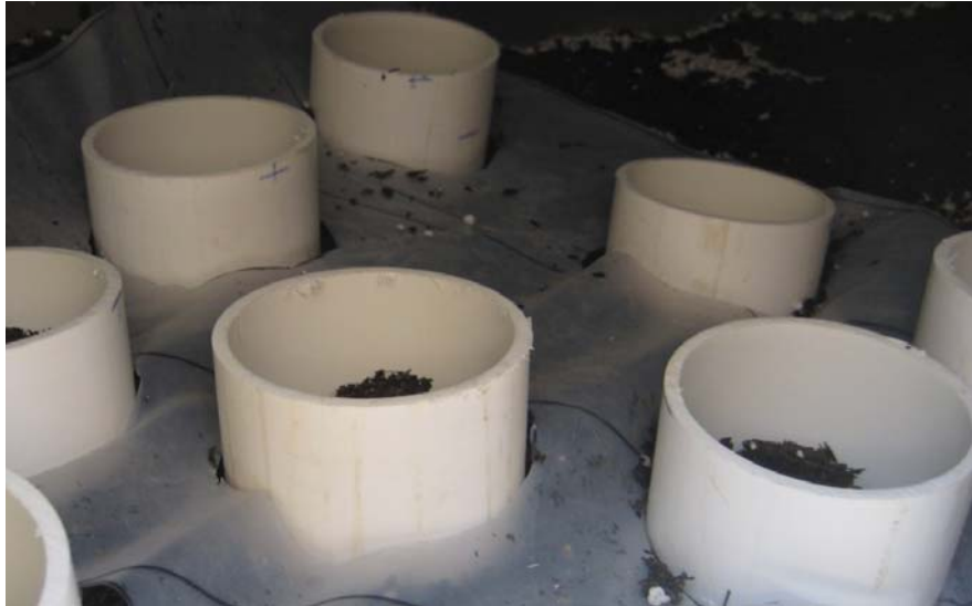
Figure 44. PVC cores forced 4” deep into each hole in the template, with collected soil
