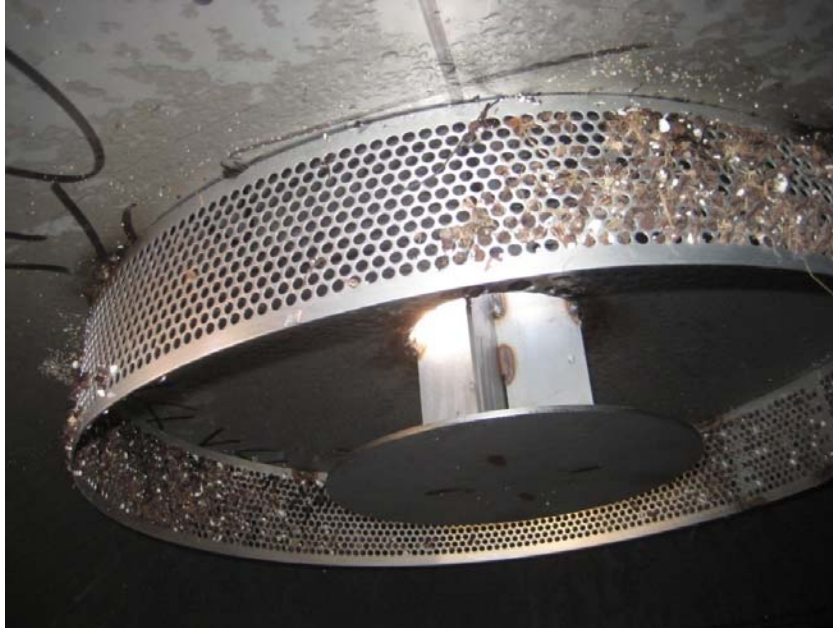
Figure 39. Potting soil caught on inlet dissipation screen of the Lakos media tank. Flow-Guard has a similar dissipation screen, but was not tested with potting soil.
