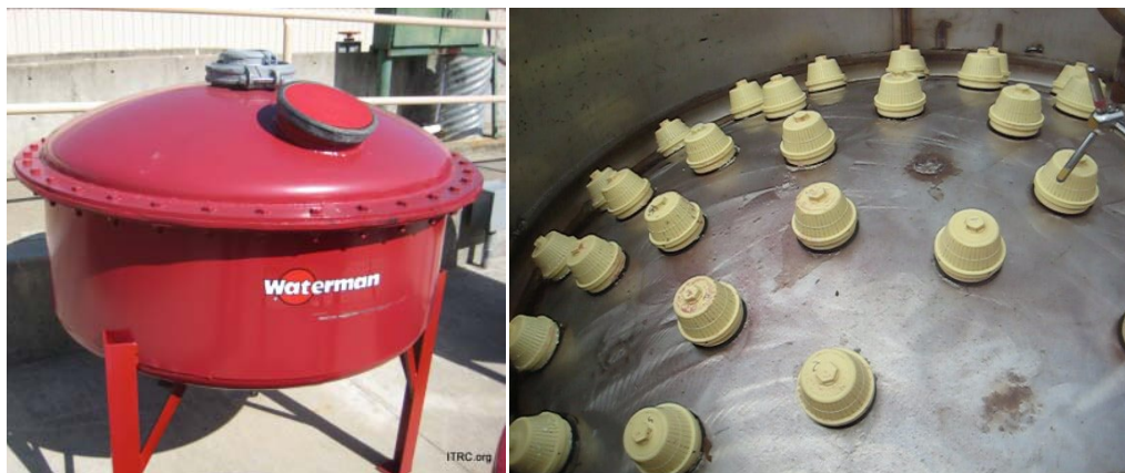
Figure 5. Waterman Dome exterior and underdrain
