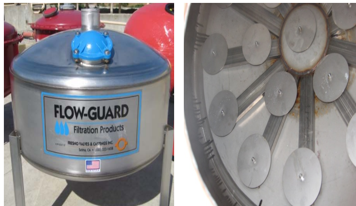
Figure 2. Flow-Guard exterior and underdrain
