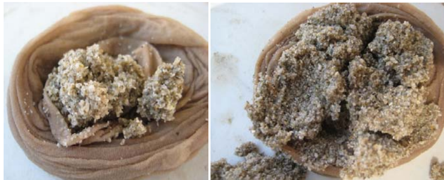
Figure 37. Examples of large amounts of media removed during backflush
